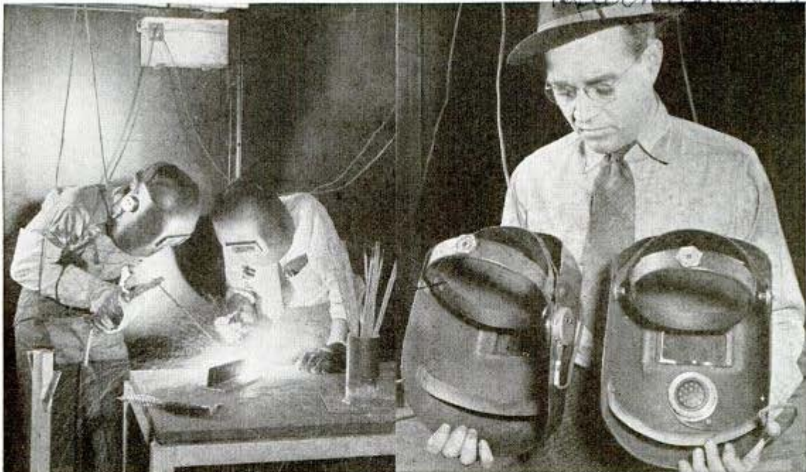
Left, apprentice and instructor using one-way phone; helmets, right, reveal receiver and transmitter
